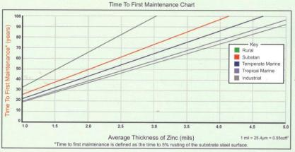
complete coverage and all of these other features, provide hot-dip galvanized steel with a long, maintenance-free service life. The time to first maintenance for hot-dip galvanized steel can be seen in this chart.
